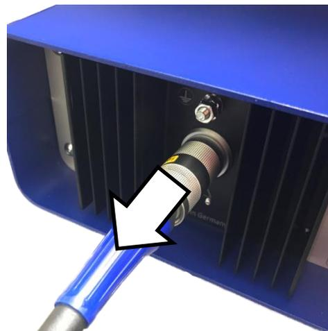
To disconnect the hand-held welding gun, pull the LEMO plug backwards. Again, no turning is necessary.
